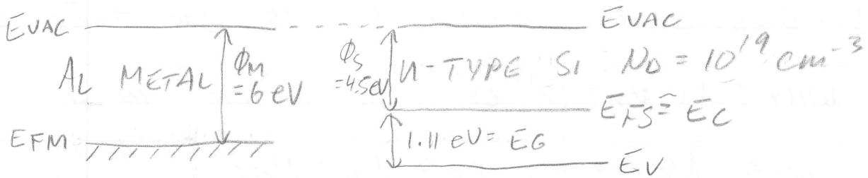
AT CONTACT, ELECTRONS WILL MOVE FROM THE Si TO THE Al, SINCE  $E_{FS} > E_{FM}$ , UNTIL AN EQUILIBRIUM IS REACHED, WITH A CONSTANT EF ACROSS THE Al AND Si:
