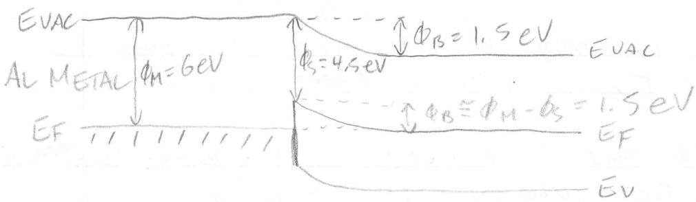
② SO THE BARRIER HEIGHT = BAND BENDING =  $\phi_B = \phi_M - \phi_S = 1.5 \text{ eV}$
